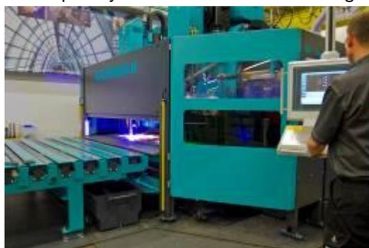
Gains from ongoing Kaltenbach software and control development have reduced processing cycle times and minimised any dwell between processes. Nesting has been further refined to achieve minimum metal waste, maximum production output, using grid or common-cut procedures.
