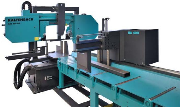
From Kaltenbach's hugely successful Mitre Bandsaw series, the KBS400 DG-NA (pictured) is a compact, bi-directional mitring machine, suitable for use in cutting sections and profiles up to 400mm wide x 350mm high. The DG-NA model includes a fully automatic material feed unit for the reliable batch production of a wide variety of straight and mitred pieces. Available also as a semi-automatic model, the machine offers excellent
