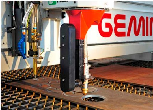
It's the most technologically advanced, small footprint CNC machining system for the profile cutting, drilling, bevelling, machining and scribing of parts from plate, from 5mm up to 120mm thick with cutting lengths from 6 to 30 metres - in just one set-up. The new compact bevelling head is now 25% lighter than similar machines and has internal kinematic making it even faster and more flexible. The scribing system can also significantly reduce fabrication time and manpower requirements.
