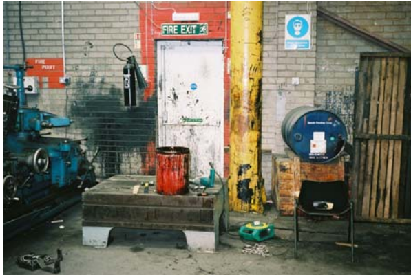
An example of poor housekeeping in a workshop – you can see that this work area is full of potential hazards.
